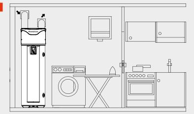
The installation of the heat pump water heater requires a omni-polar circuit-breaker of 16 A and a earth leakage trip of 30 mA not given as standard with RAPAX V2.
