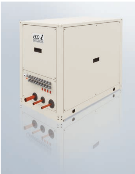
Panasonic offers a purposely engineered solution which allows for a quick and simple installation. The unit contains 5 actuating ball valves, a 30l storage vessel and PLC all housed in an IP54 rated container. Terminals on the front of the unit allow for easy wiring to the alarm terminal, high / low pressure transducers and discharge temperature sensor(s) of the condensing unit(s).
